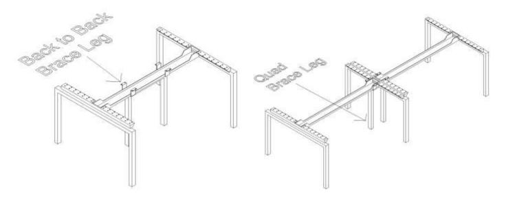
**Note**: When return work surfaces are utilized brace legs are not necessary.
