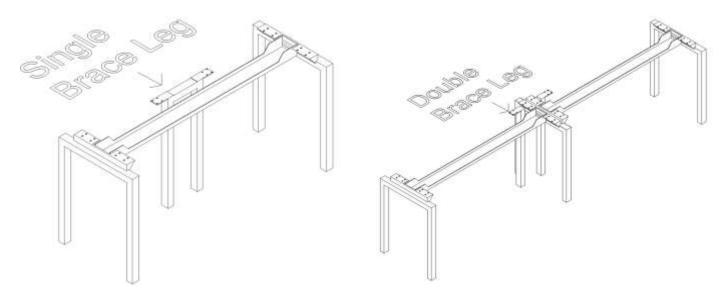
**Note**: When return work surfaces are utilized brace legs are not necessary.
