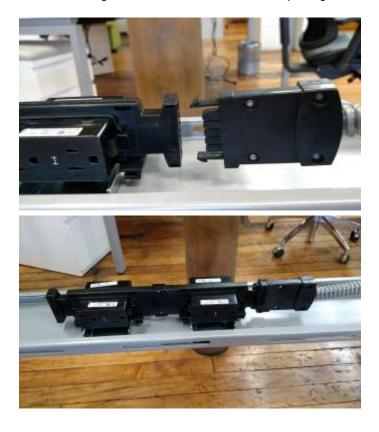
When power bars are in the desired location install the 4 securing screws that came with the cable tray.
