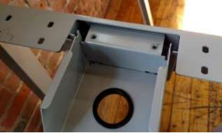
After inserting the teeth, the cable tray must be pushed down to lock the teeth into the leg (a rubber hammer may be used to assist). Re-install the two hole plate and tighten the screws to fully secure the cable tray.
